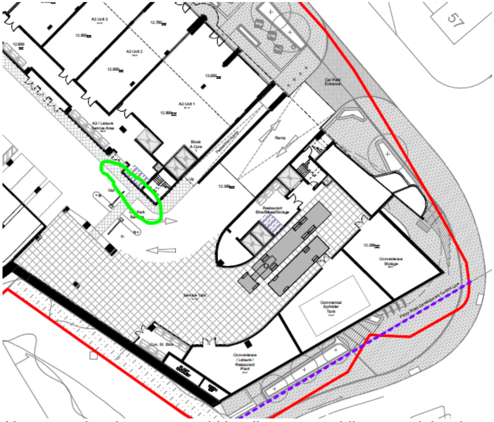
Narrow pedestrian access width adjacent to public car park barriers
